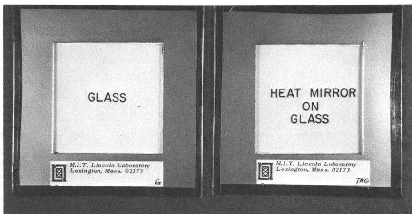
Figure 8. Photographs of a bare glass substrate (Corning 7059 glass) and of a similar glass substrate coated with a 330-Å \text{TiO}_2 /130-Å \text{Ag}/330\text{-Å} \text{TiO}_2 film
